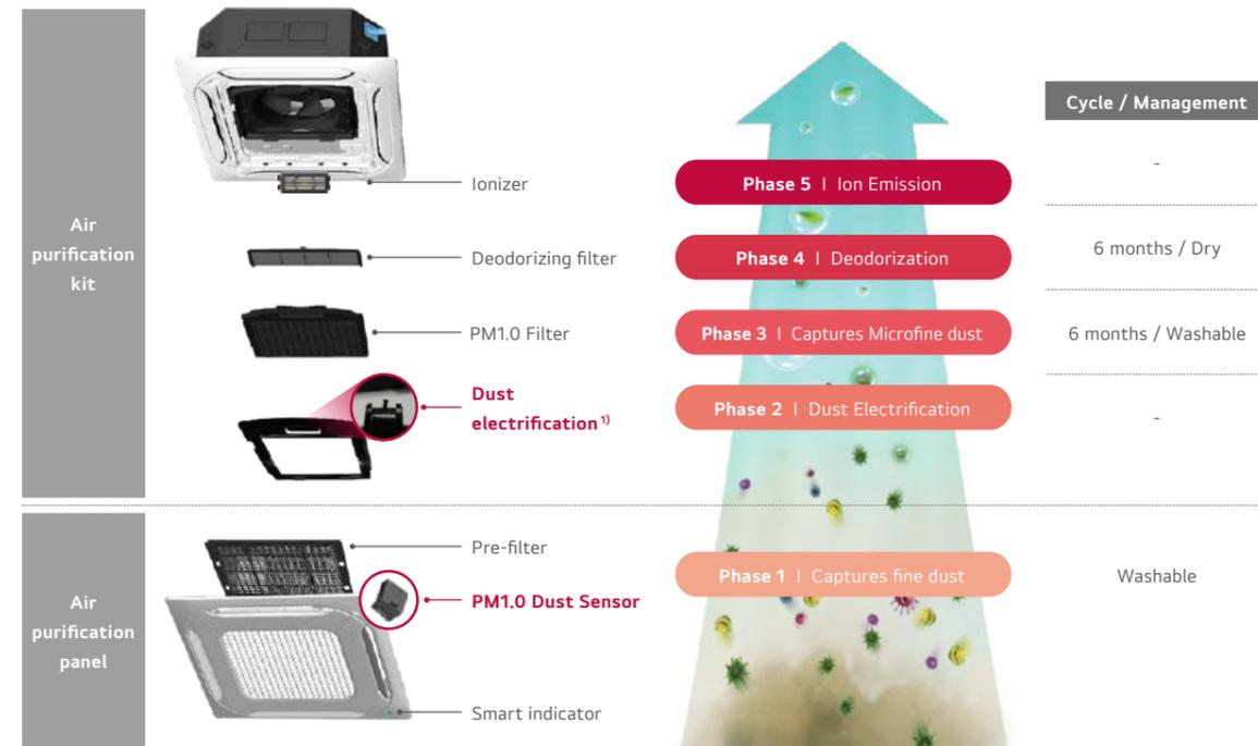
1) Electrical diffusion makes dust electrification.
