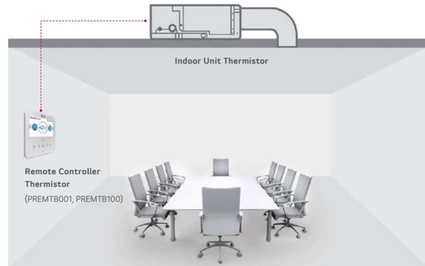
Compares temperatures sensed from different positions, and automatically selects the optimum temperature for users.
