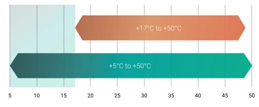
EWT range in cooling at nominal water flow (°C)
