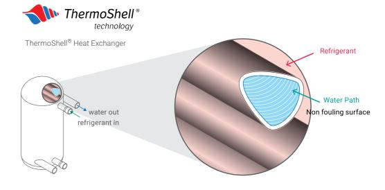
Coaxial Heat Exchanger
