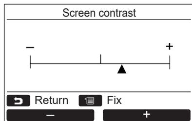
**1** Push the [ ] / [ ] button to select “3.Screen contrast” on the “Initial setting” screen, then push the “ Set” [F2 F2] button.
