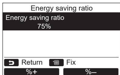
**1** Push the [ ] / [ ] button to select “2. Energy saving ratio” on the “Energy saving operation” screen, then push the “ Set” [ F2] button.
