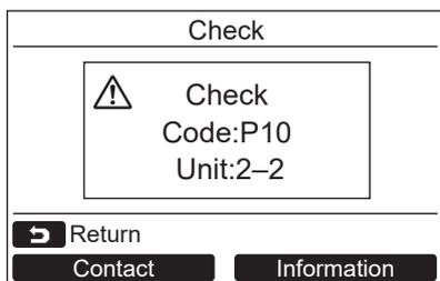
While the check information screen appears: Push the “Contact” [F1] button to display the contact number for service.
