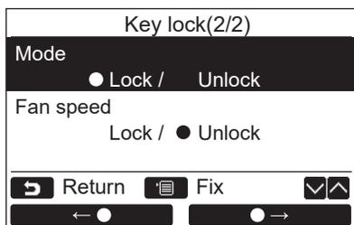
**1** Push the [ ] / [ ] button to select “5 Key lock” on the “Initial setting” screen, then push the “ Set” [F2] F2] button.
