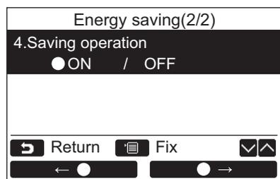
**1** Push the [ ] / [ ] button to select “4. Saving operation” on the “Energy saving setting” screen, then push the “ Set ” [F2 F2] button.
