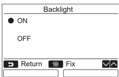
**1** Push the [ ] / [ ] button to select “4.Backlight” on the “Initial setting” screen, then push the “ Set” [F2] F2] button.
