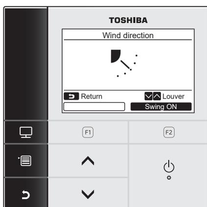
**1** Push the [ ] / [ ] button to select "1. Wind direction" on the menu screen, then push the " Set" [ F2 ] button.
