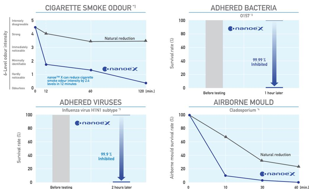
\*1 <Cigarette smoke odour> [Test organisation] Panasonic Product Analysis Centre [Test method] Verified using the 6-level odour intensity scale method in an approximately 23m<sup>3</sup> sized test room [Test method] nanoe™ released [Test substance] Surface-attached cigarette smoke odour [Test result] Odour intensity reduced by 2.4 levels in 12 min. [4AA33-160615-N04]
