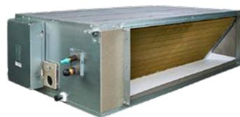
**The indoor unit** has a fan coil which conditions the supplied air, this conditioned air is then distributed through ducting in the roof to outlets in ceiling or walls.
