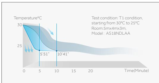
With the Turbo function the motor and fan work at a higher frequency, so you can enjoy a cool room within a much shorter time.
